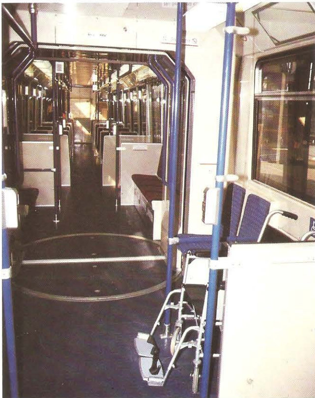
The spacious interior provides ample room for standing passengers and the wide vestibule by the articulation enables them to move freely through the vehicle.
