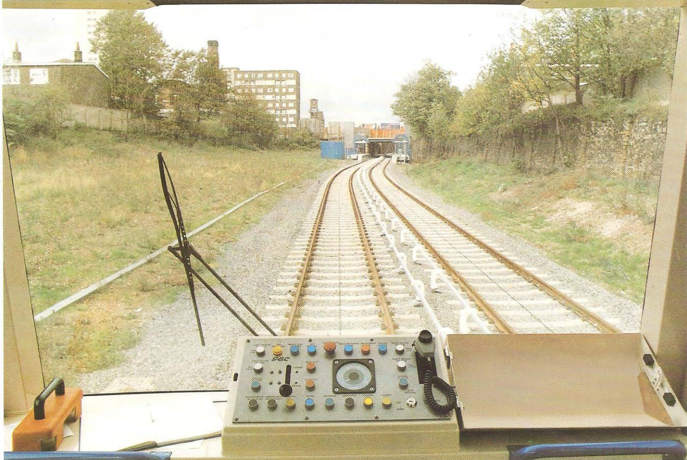
The trains can be operated from an Emergency Driving Position (EDP) at each end of the vehicle. Normally the EDP is covered by a locked lid and is used only in the depot area or if there is an equipment failure.
