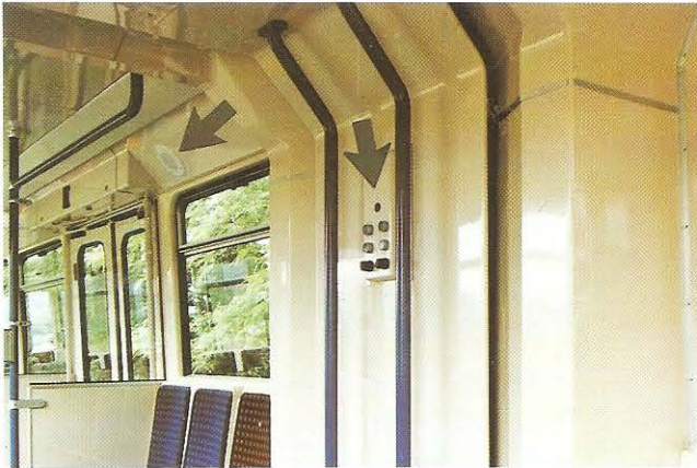
The train captain can speak to his passengers using the on-board public address system located on the articulation section whilst his door controls are located above each doorway.
