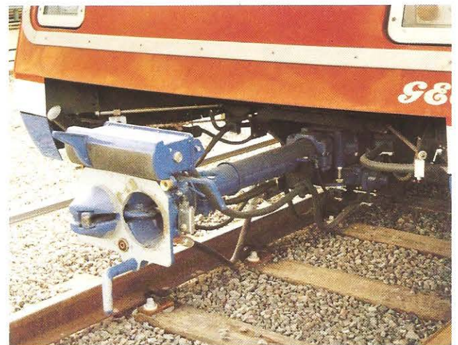
Autocouplers provide pneumatic and multiple electrical connections between vehicles as well as mechanical.
