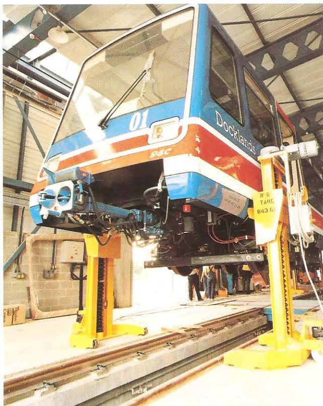
Part of the workshop section of the OMC showing a vehicle jacked-up during commissioning.
