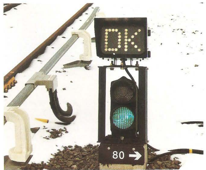
Fibre optic indicators and ground signal at the exit from the OMC.
